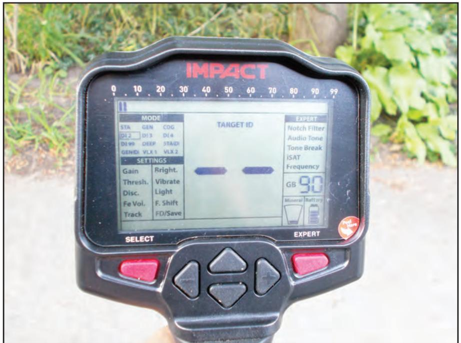
*The Impact's screen provides easy access to all of its features without complicated menus. Real-time information on ground condition, battery strength, and target composition are also shown on the screen. Backlighting allows it to be used in low and no-light conditions.*
